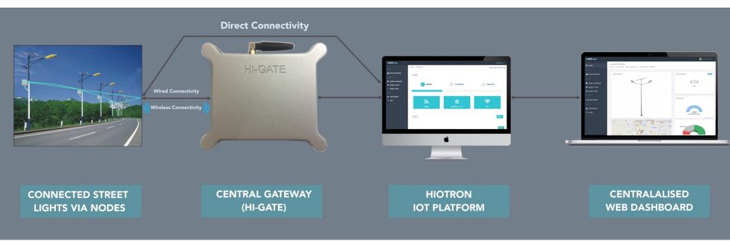
hIOTron offer three Node – Gateway connectivity solutions such as Wired, Wireless & gateway as Node for street light remote control and status data transmission.
