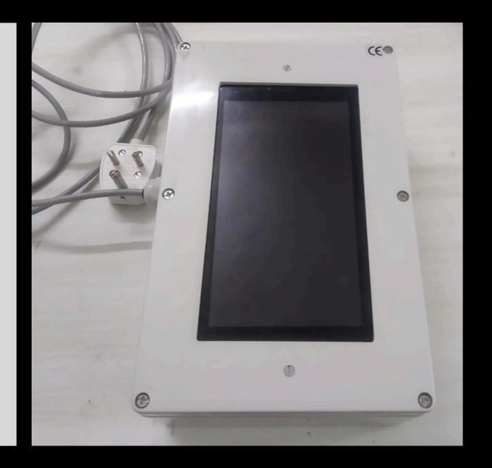
• DIOT Box – DIOT Box is compact version of DI & IOT box act as a standalone Industry4.0 gateway which collect data from machines via PLC in digital format and processes that data in real-time, store in local memory and streams data securely to the hIOTron Industrial IoT platform using Wi-Fi, Ethernet & GSM (optional).
